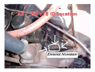
Studebaker V8 engine: The Studebaker V8 was developed in-house in 1949-50 by the Studebaker engineering department under the direction of Stanwood W. Sparrow. It was available in different displacements at different times. Although some running changes were made during the period 1951-64 (e.g., converting to full-flow oil filter in mid-1962), all Studebaker V8s are essentially interchangeable, with the only major differences being bore and stroke.
